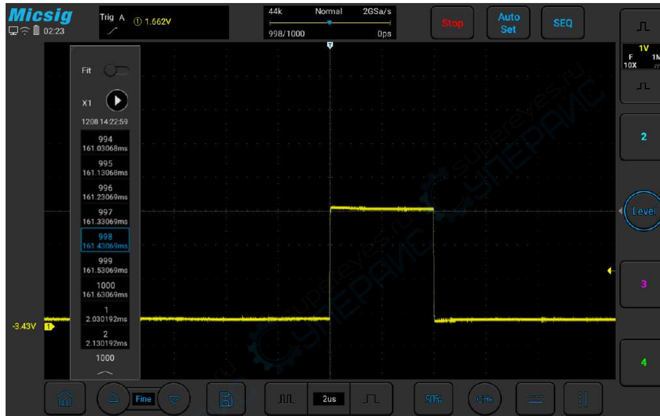
Figure 10-12 Single frame view of segmented storage
