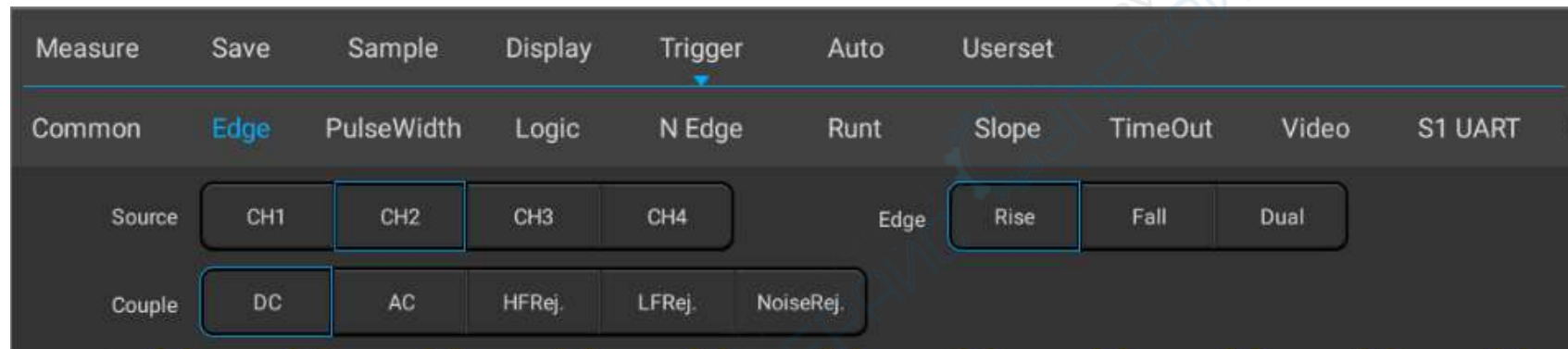
Figure 5-12 Edge Trigger Setting Menu
