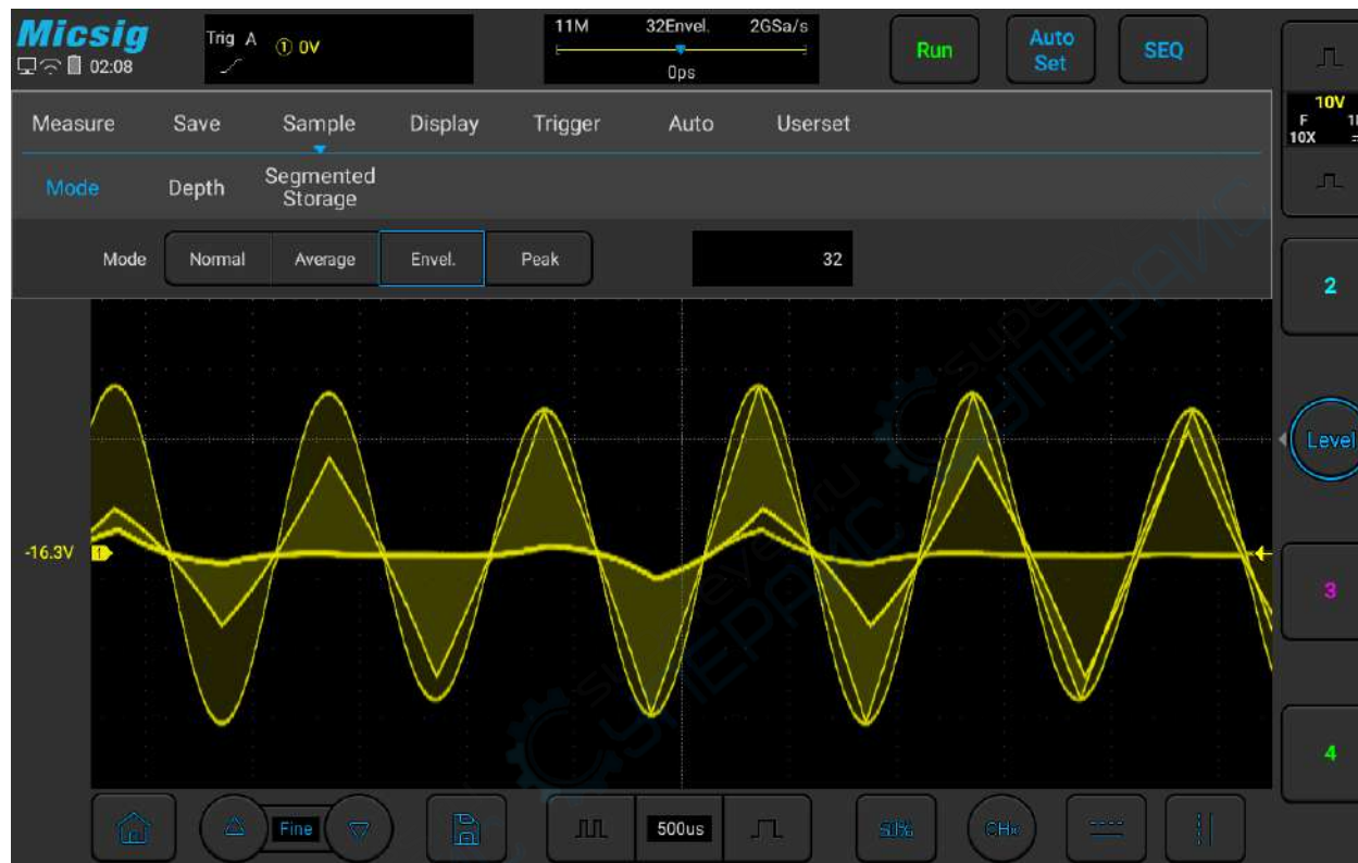
Figure 10-8 AM Signal in Envelope Sampling Mode (32)
