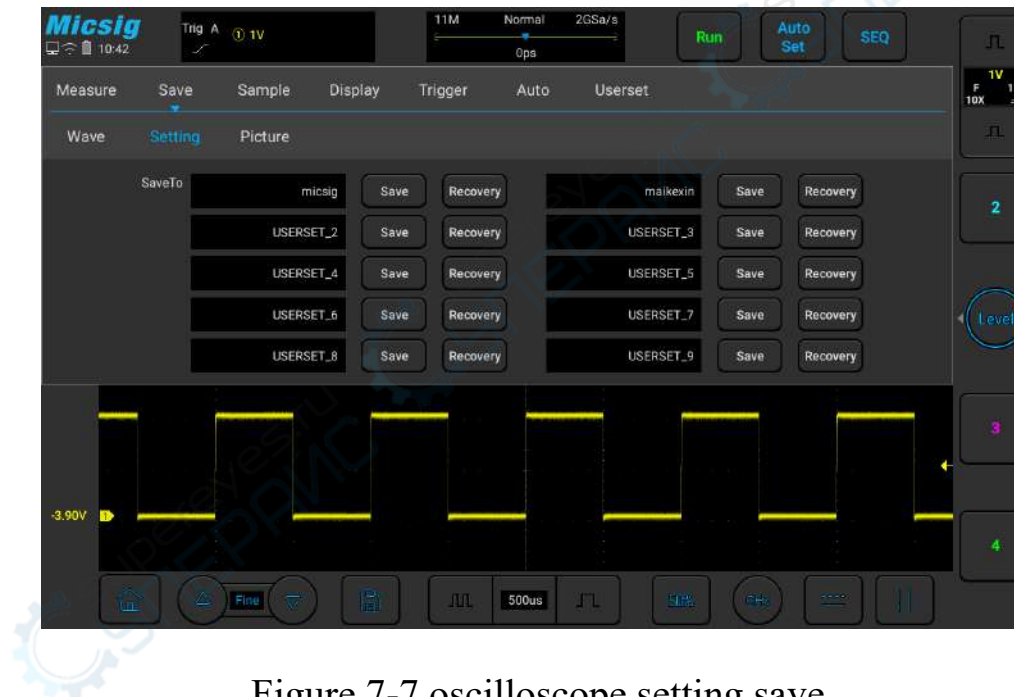
Figure 7-7 oscilloscope setting save
