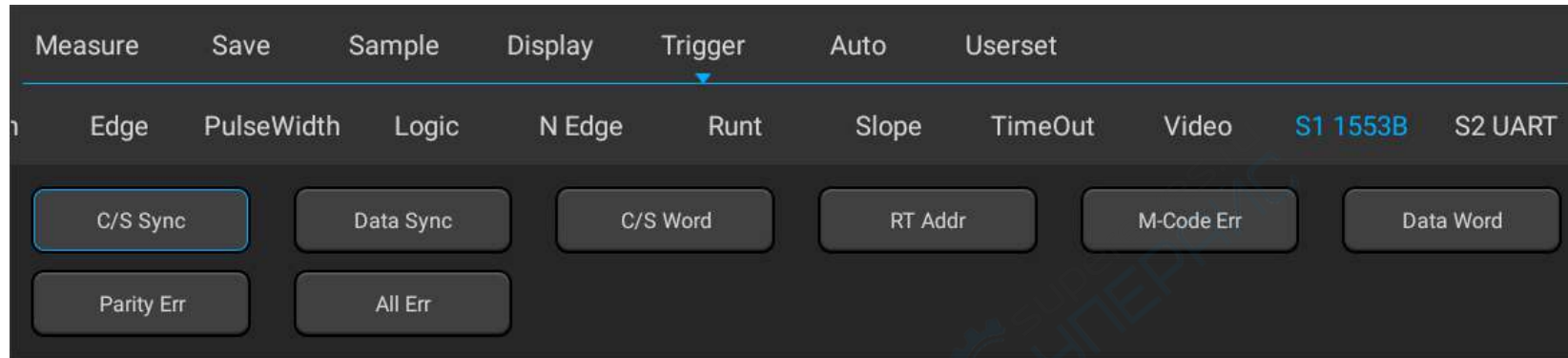
Figure 11-31 1553B Trigger Mode Configuration Menu
